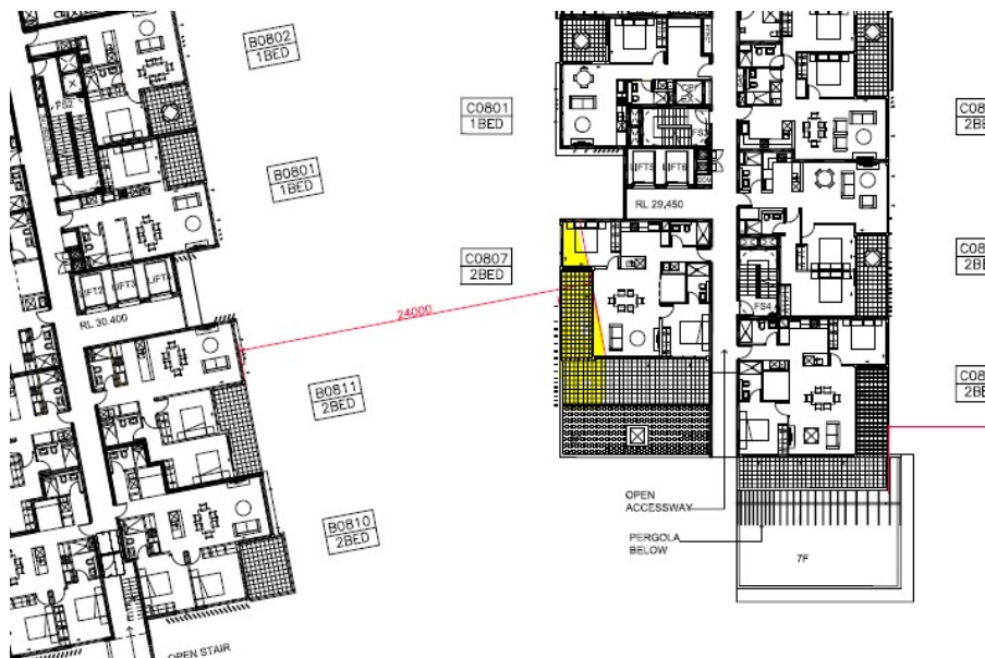
Figure 10 - Non-compliant building separation between Building B & Building C and Levels 8 & 9 (non-compliant portion highlighted yellow).
